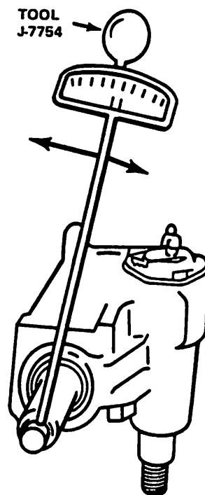
Fig. 2K-17 Adjusting Pitman Shaft Overcenter Drag Torque
