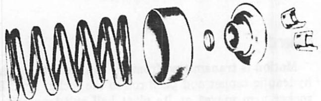
Fig. 1B-8 Valve Spring Assembly
