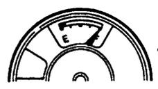
REPAIR CLUSTER GROUND OR REPLACE CVR (INTEGRAL WITH TEMPERATURE GAUGE)
