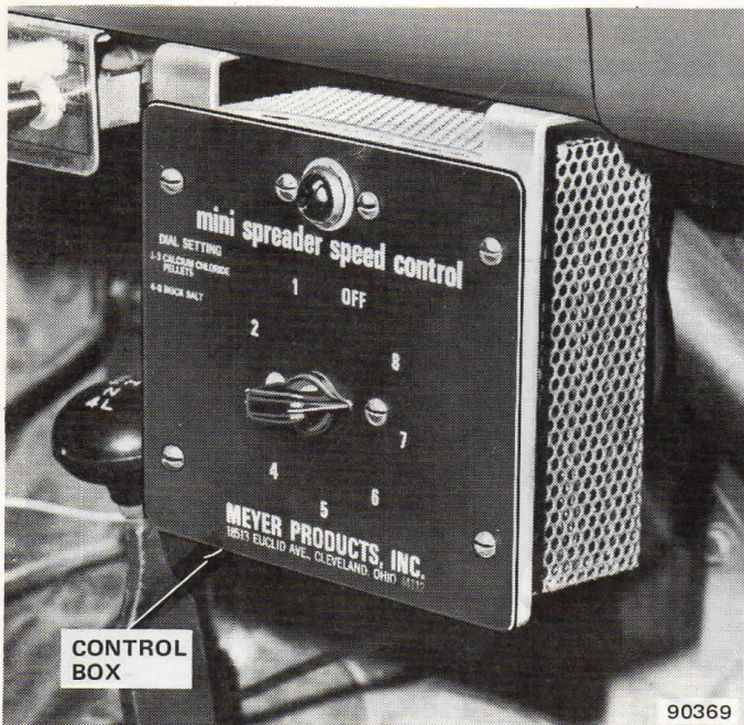
Fig. 4-7 Speed Control Box Installation
