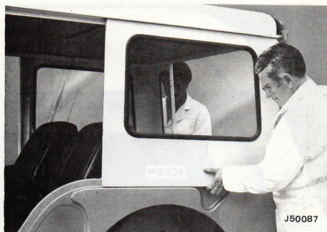
Fig. 2-19 Mounting Roof—Quarter Panel Assembly on Body
