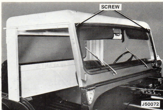
Fig. 2-4 Roof/Rear Panel Assembly Installed—Front View
