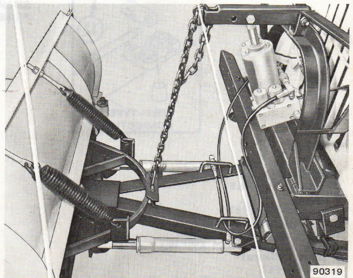
Fig. 1-18 Electronic Power Pack Models E-46 and E-47 Installations
