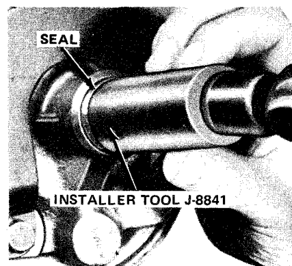
Fig. 2L-49 Pump Shaft Seal Installation
