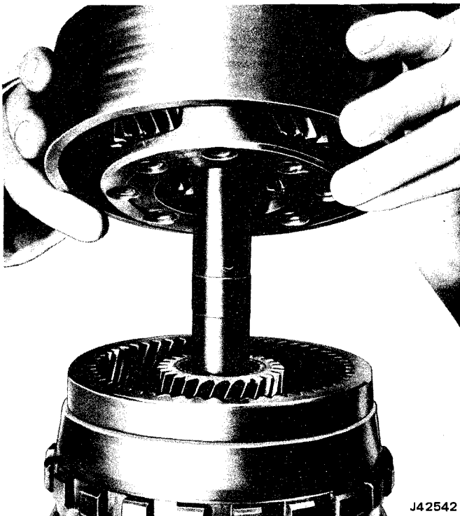
Fig. 2C-141 Reaction Carrier Installation
