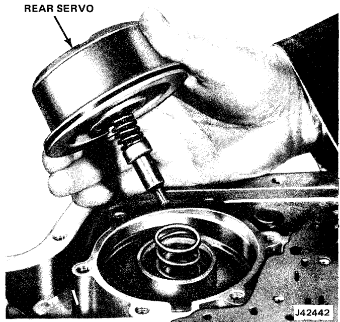
Fig. 2C-19 Rear Servo Removal-Installation
