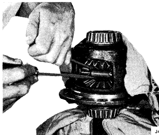
Fig. 2F-62 Pinion Mate Shaft Snap Ring Removal
