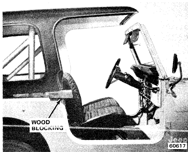
Fig. 3C-2 Hardtop Enclosure Supported with Wood Blocking
