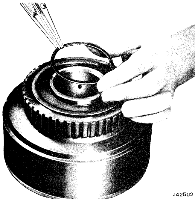
Fig. 2C-84 Intermediate Roller Clutch Snap Ring Removal
