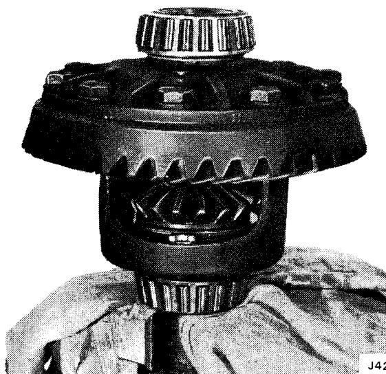
Fig. 2F-61 Differential Mounted on Axle Shaft
