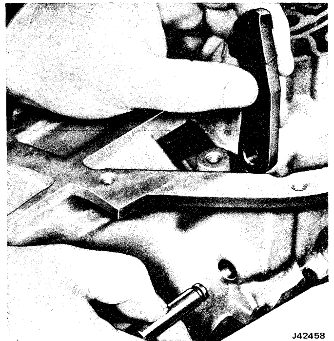
Fig. 2C-35 Parking Pawl and Shaft Removal
