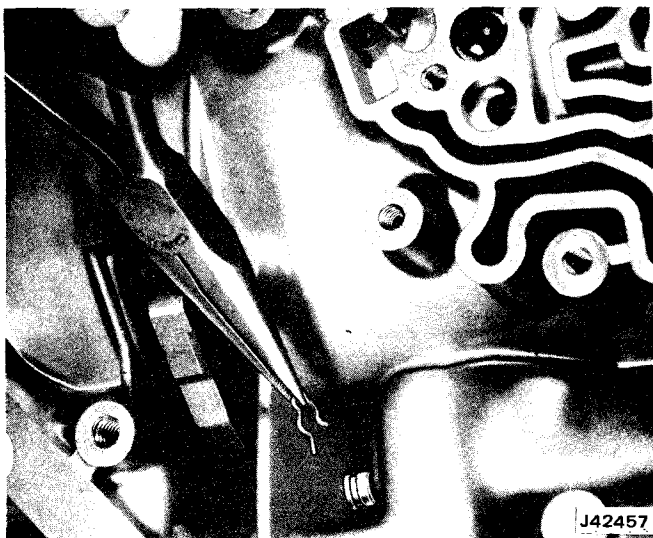
Fig. 2C-33 Parking Pawl Shaft Retainer Spring Removal-Installation
