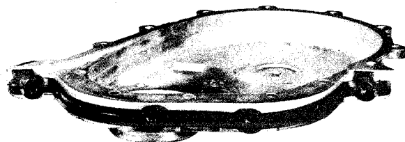
Fig. 1B-21 Oil Pan Front Seal Installation AJ41894
