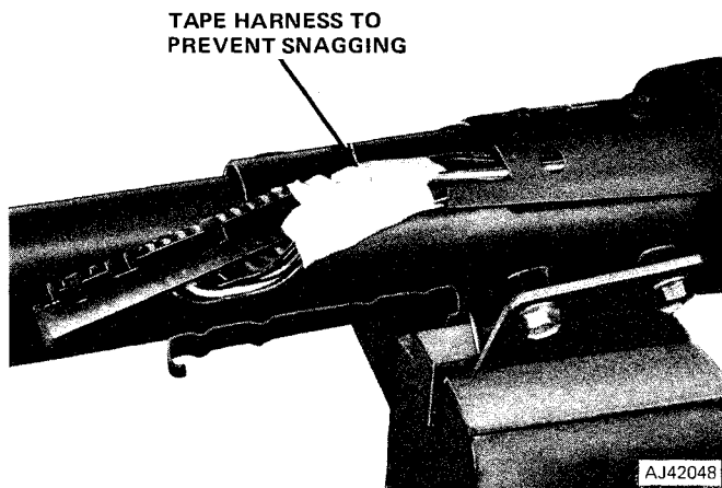
Fig. 2J-26 Turn Signal Switch Harness Removal
