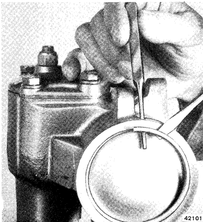
Fig. 2L-13 End Plug Retaining Ring Removal
