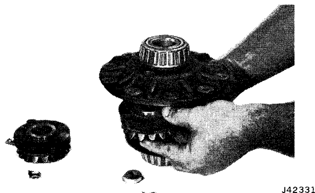
Fig. 2F-67 Side Gear and Clutch Pack Removal
