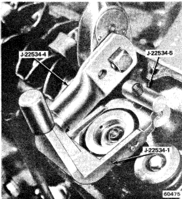
Fig. 1B-69 Valve Spring Removal
