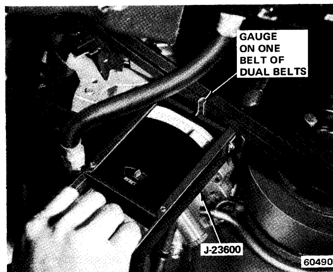
Fig. 2-13 Checking Drive Belt Tension—V-8 Engine with Air Conditioning
