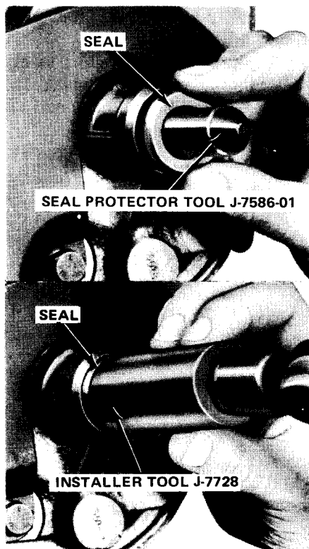
Fig. 11-98 Installing Pump Shaft Seal
