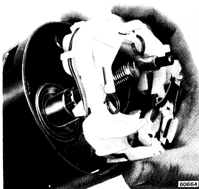
Fig. 11-8 Removing-Installing Turn Signal Switch
