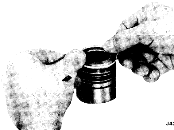
Fig. 11-87 Installing Valve Seal Rings
