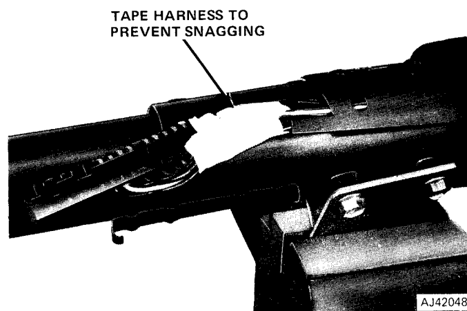
Fig. 11-29 Signal Switch Harness Removal
