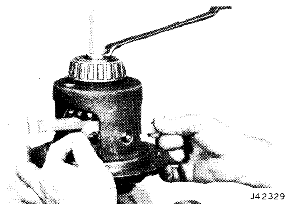
Fig. 10-69 Removing Pinion Thrust Washer
