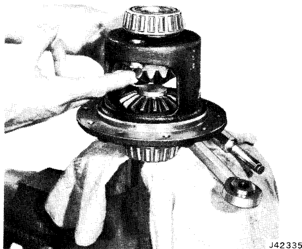
Fig. 10-74 Installing Clutch Pack and Side Gear
