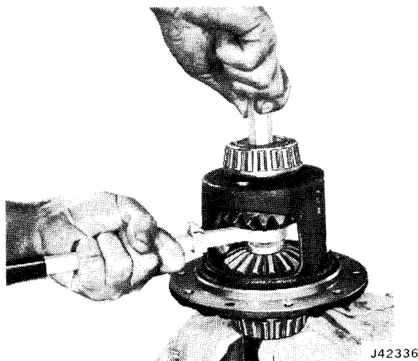
Fig. 10-75 Threading Forcing Screw into Rotating Tool
