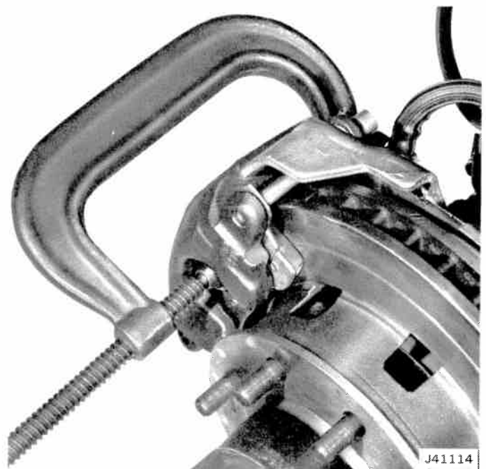
Fig. 9-39 Bottoming Piston with C-Clamp
