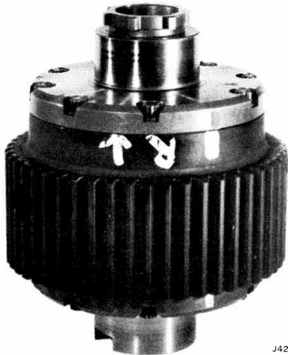
Fig. 8-49 Case Sprocket and End Caps Identified for Orientation
