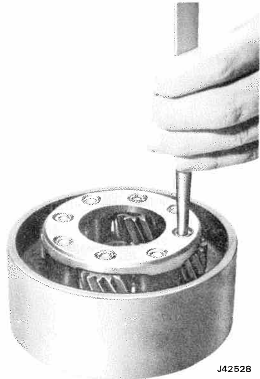
Fig. 7-98 Removing Planet Pinion Pins
