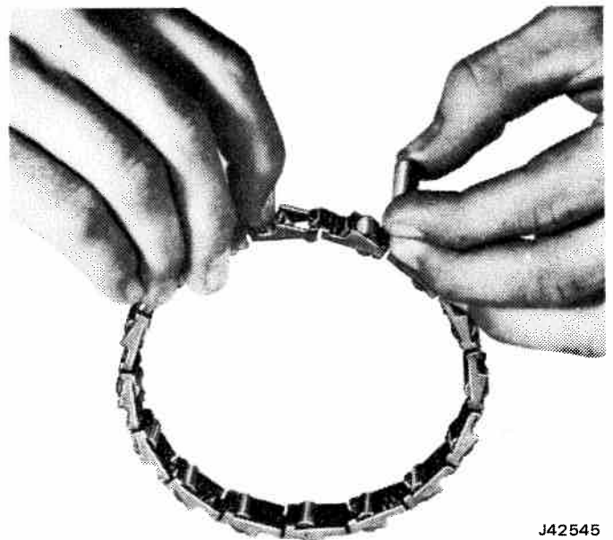
Fig. 7-115 Installing Roller in Roller Clutch
