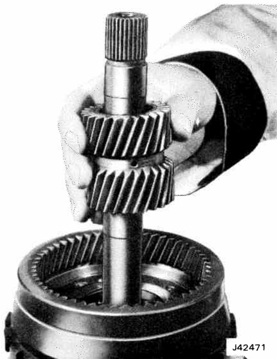
Fig. 7-41 Removing Sun Gear
