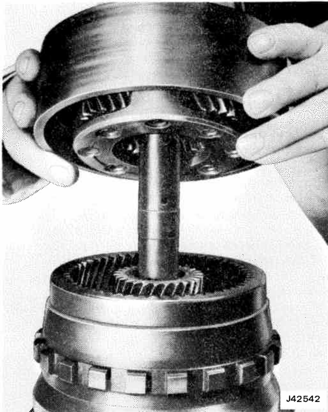
Fig. 7-112 Installing Reaction Carrier Assembly
