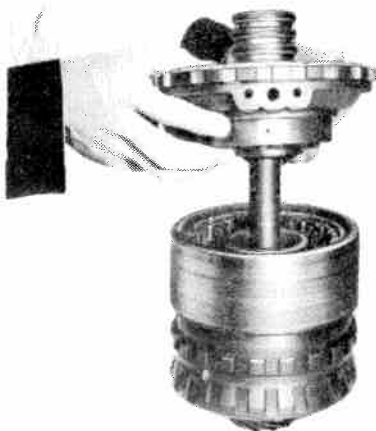
Fig. 7-117 Installing Center Support
