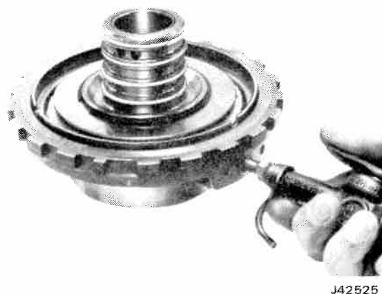
Fig. 7-95 Checking Operation of Intermediate Clutch Assembly
