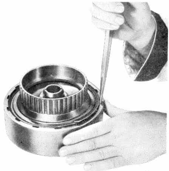
Fig. 7-61 Removing Forward Clutch Housing Snap Ring
