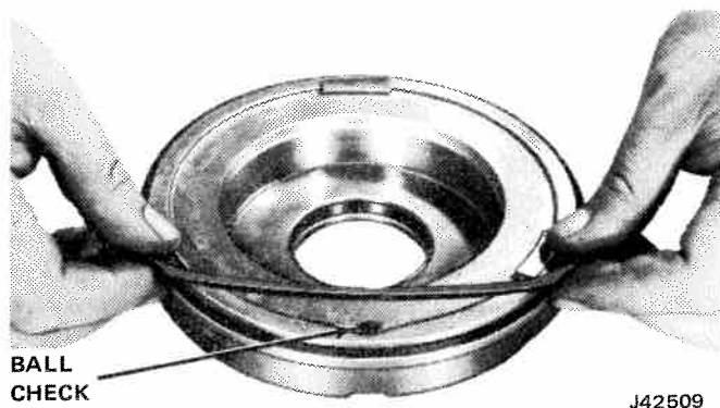
Fig. 7-79 Installing Outer Seal on Direct Clutch Piston
