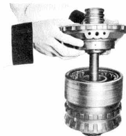
Fig. 7-38 Removing Center Support from Gear Unit
