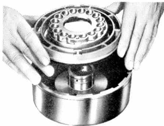
Fig. 7-77 Removing Piston From Direct Clutch Housing
