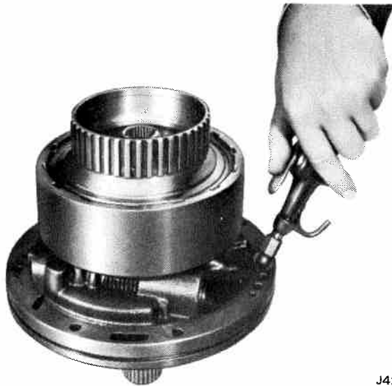
Fig. 7-71 Checking Forward Clutch Operation
