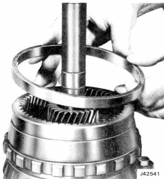
Fig. 7-111 Positioning Front Internal Gear Ring
