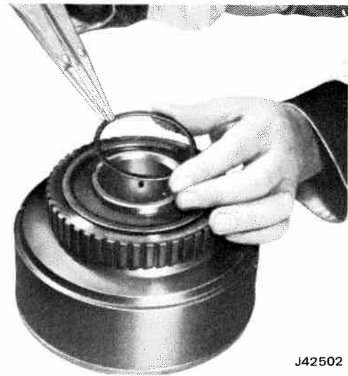
Fig. 7-72 Removing Intermediate Clutch Roller Snap Ring
