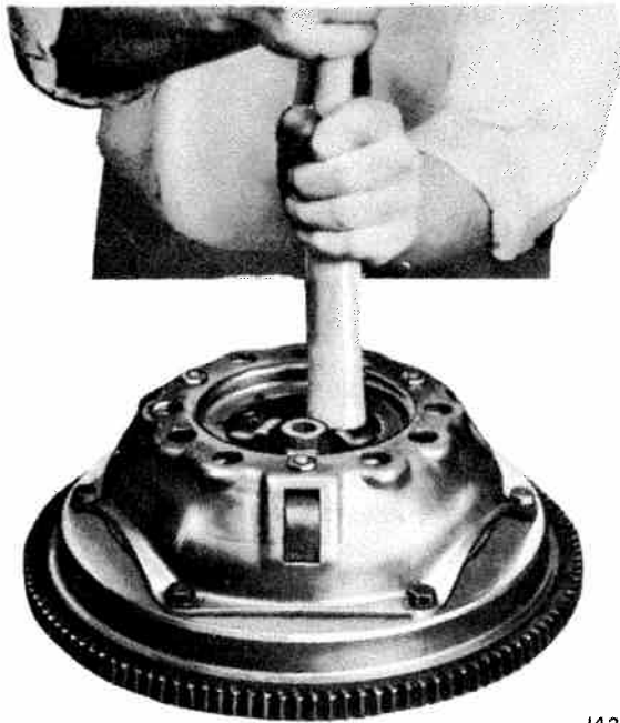
Fig. 5-7 Depressing Clutch Levers
