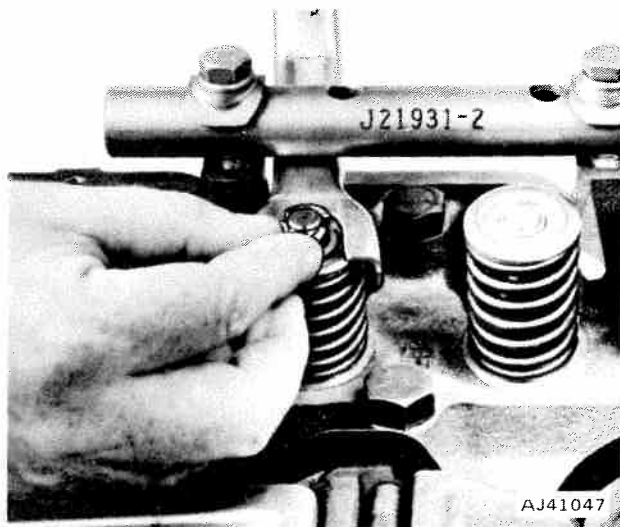
Fig. 1A-10 Valve Spring Removal
