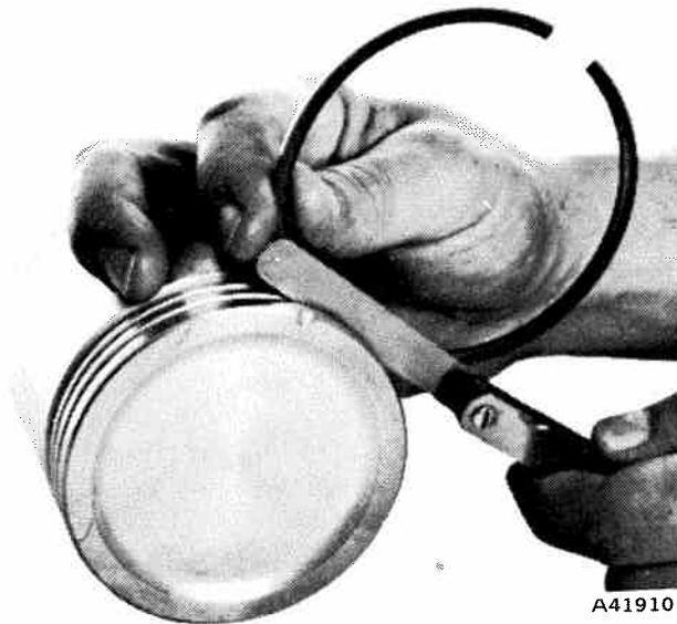
Fig. 1A-40 Ring Side Clearance
