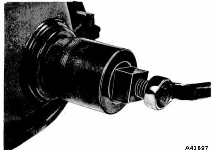
Fig. 1A-27 Timing Chain Cover Oil Seal Removal
