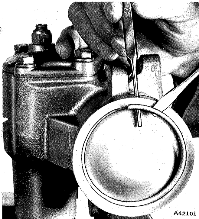
Fig. 2L-13 End Plug Retaining Ring Removal
