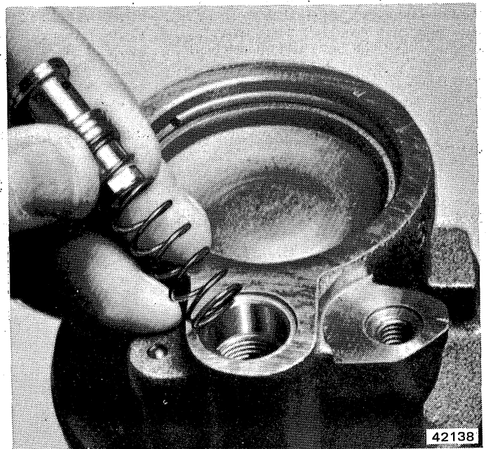
Fig. 2L-61 Flow Control Valve and Spring Installation
