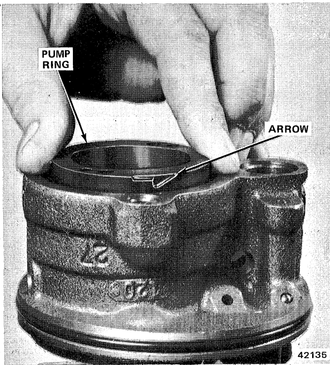
Fig. 2L-58 Pump Ring Installation
