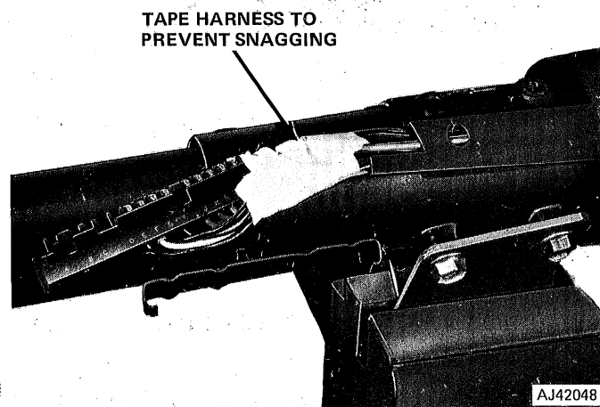
Fig. 2J-27 Turn Signal Switch Harness Removal
