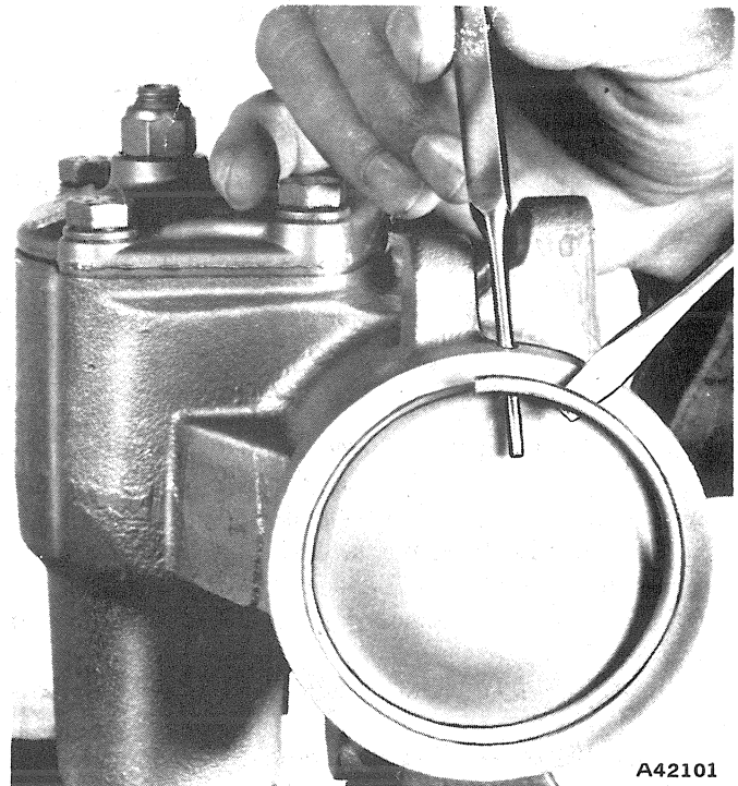
Fig. 2L-13 End Plug Retaining Ring Removal
