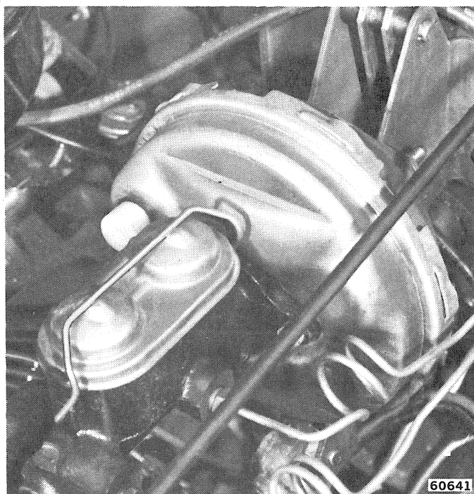
Fig. 2G-21 Power Brake Unit and Bellcrank—CJ Models
