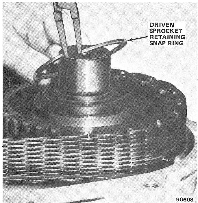
Fig. 2D-13 Driven Sprocket Retaining Snap Ring Removal/Installation
