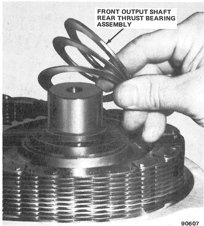
Fig. 2D-12 Front Output Shaft Rear Thrust Bearing Assembly Removal/Installation
