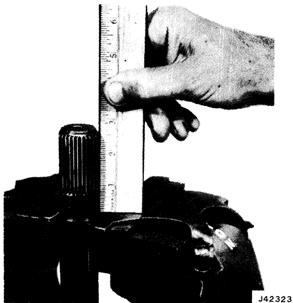
Fig. 10-59 Axle Shaft Positioned in Vise
