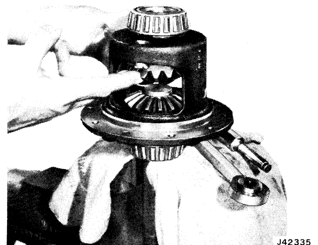
Fig. 10-69 Installing Clutch Pack and Side Gear
