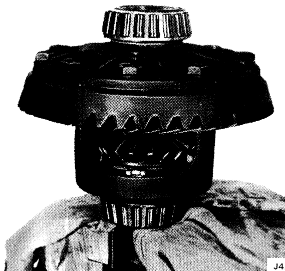
Fig. 10-60 Differential Mounted on Axle Shaft
